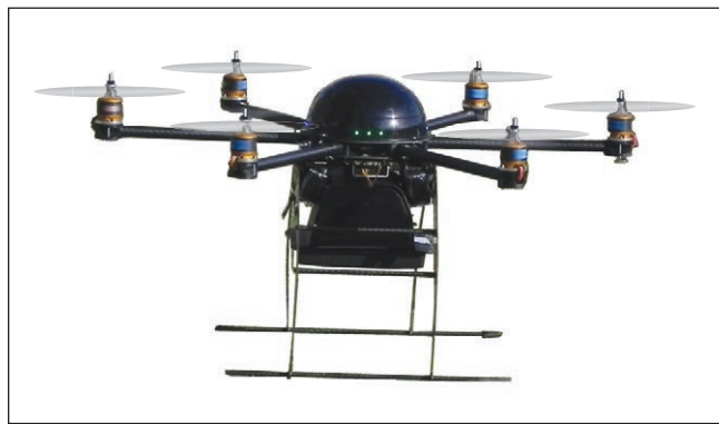
▲ Fig. 2 TiaLinx mini UAV, including radar sensors for-through-the-wall imaging (photo courtesy of TiaLinx).
