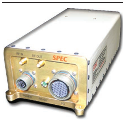
▲ Fig. 2 Agile Digital Effects Processor Digital RF memory unit.
