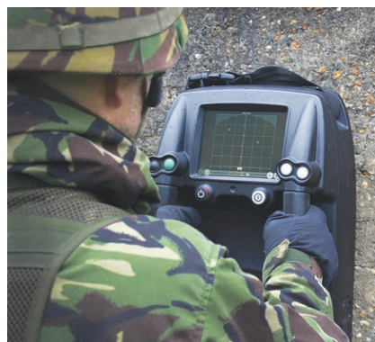
▲ Fig. 4 Cambridge Consultants' through-the-wall radar sensor unit (photo courtesy of Cambridge Consultants).
