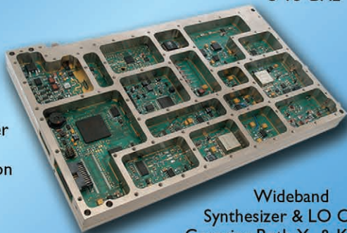
Amplified Switch Filter Bank 9 Selectable Bands 5-18 GHz
